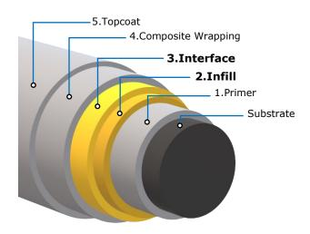
Corro-Dur™ 450 can be used as Infill/ Rebuilding and Interface Agent for Composite Wrapping
